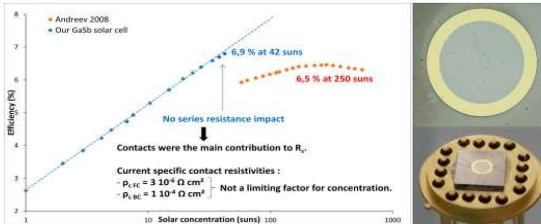
**Figure 1:** (Left) Efficiency versus solar concentration for the current GaSb concentration record and our own GaSb solar cell.
