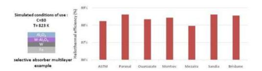
Heliothermal efficiencies of selective thermooptical multilayers optimized using ASTM solar spectrum reference and local spectra (case of W/W-Al<sub>2</sub>O<sub>3</sub>/Al<sub>2</sub>O<sub>3</sub> selective multilayer used at C = 80 and T = 823 K)
