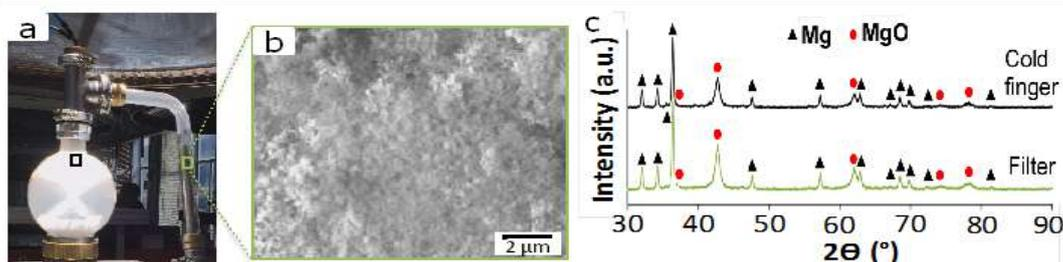
**Figure 1.** (a) "Héliotron" reactor during an experiment, (b) micrograph and (c) XRD patterns of the powder collected on the filter after a carbothermal reduction of MgO
