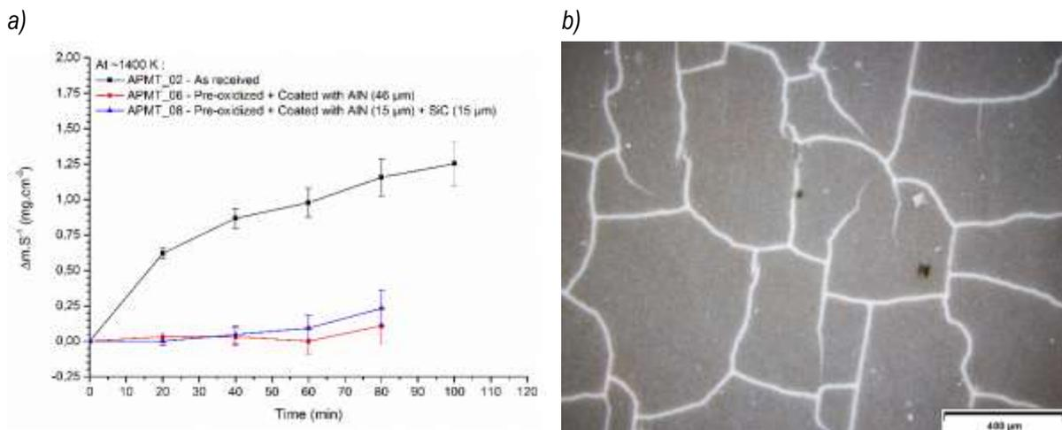
**Figure 1.** Evolution of the mass change after several cycles of 20 min. oxidation in air at 1400 K (a), and optical picture of AlN/SiC coated Kanthal APMT after 3 cycles of 20 min. oxidation in air at 1400 K (b)
