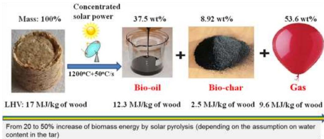
Figure 1. Experimental energy balance of wood solar pyrolysis
