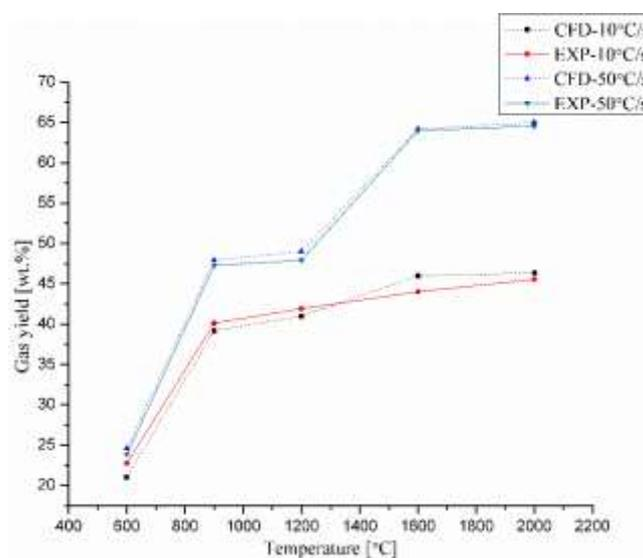
Figure 2. Gas yield comparison between the CFD model prediction values and experimental results
