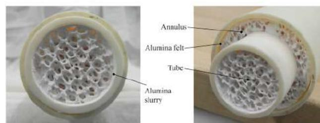
**Figure 1:** Tubular exchangers garnished with alumina foam
