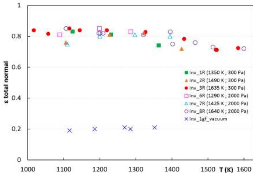
Evolution of the total normal emissivity versus temperature for the non-oxidized Inv\_1gf sample measured in high vacuum and for several pre-oxidized Invar samples (Inv\_xR) at 300 and 2000 Pa in air plasma conditions
