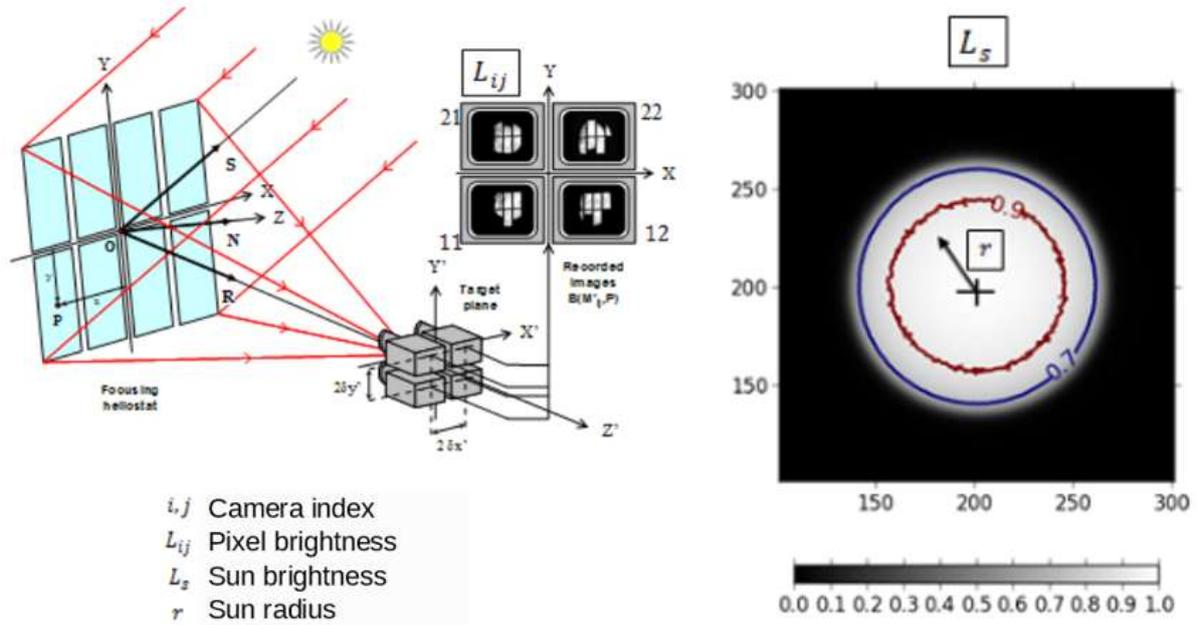
**Figure 1:** Backward-gazing method principle (left) and Sun characterization by the fifth camera (right).
