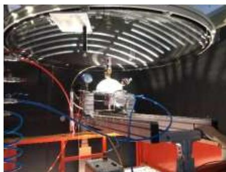
**Figure 1.b.** Photo of the solar pyrolysis reactor
