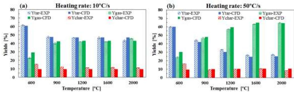
**Figure 2.** Comparison of experimental and simulation results (gas, tar and char yield as a function of pyrolysis temperature)
