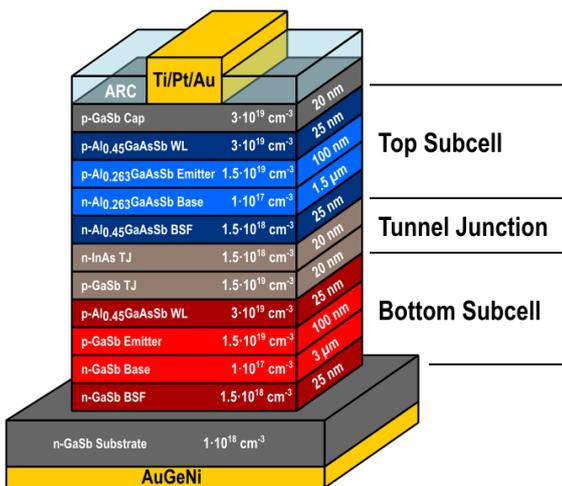
Figure 1: Architecture de la cellule tandem AlGaAsSb/GaSb
