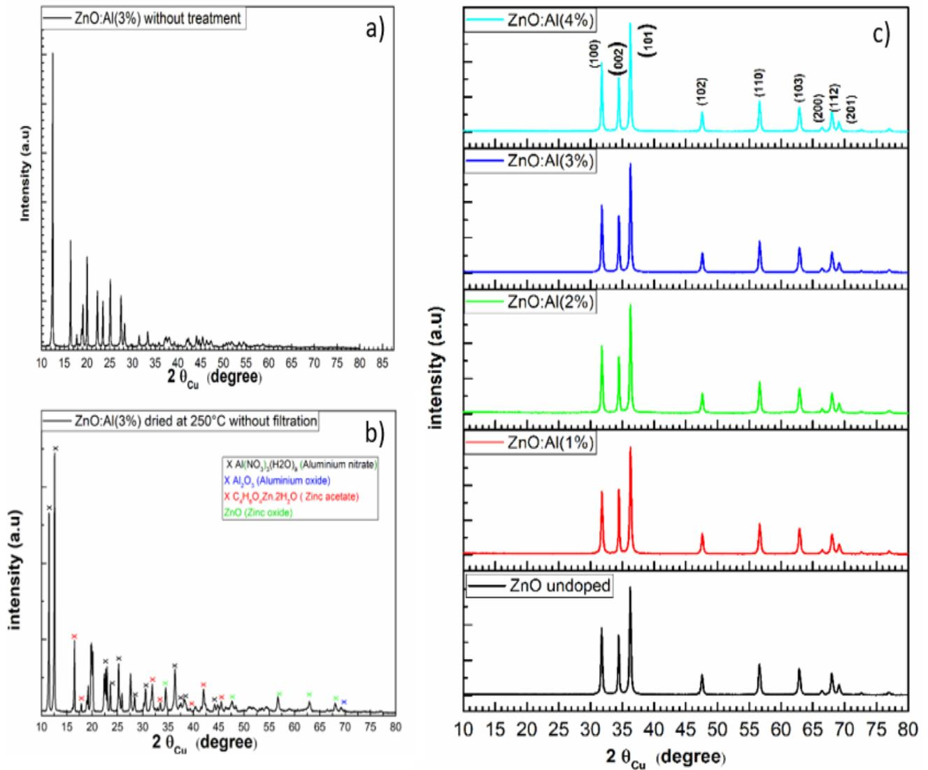
**Figure 1:** X-ray patterns of doped ZnO NPs, (a) NPs of ZnO:Al (3%) without any treatment, (b) NPs of ZnO:Al (3%) after a thermal annealing, without a filtration step and (c) NPs of ZnO:Al with varied Al doping ratio after a filtration and thermal annealing steps.
