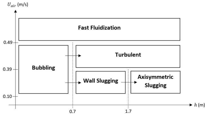
**Figure 1:** Diagram of the fluidization regimes encountered in the tube and their transitions depending on the tube height and the air velocity.
